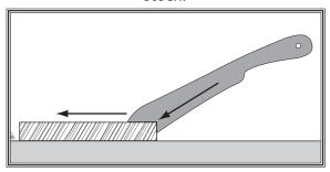
Figure 70. Side view of push stick in-use.
